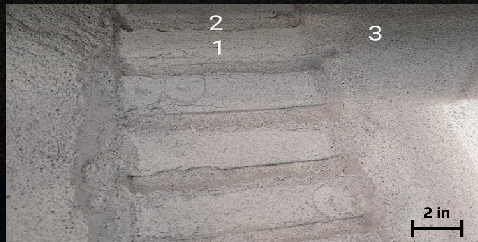
Figure 3: Temperature collection locations (numbered 1, 2, and 3) for wheel passes 1-10
