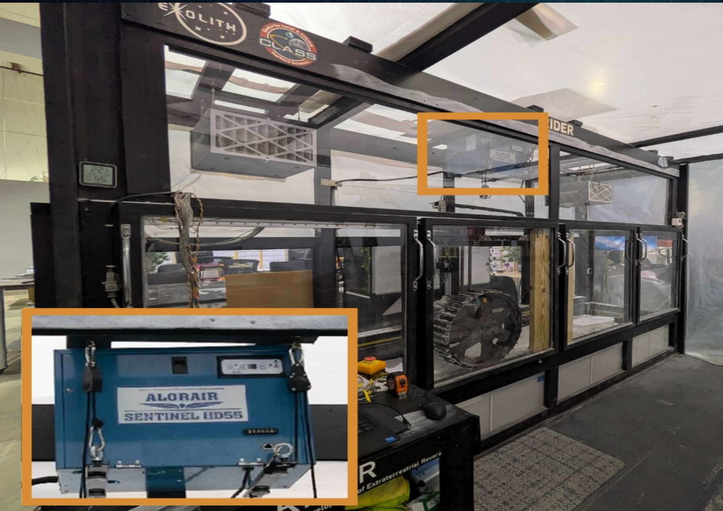
Figure 1: RIDER facility at UCF's Exolith Lab, with dehumidifier unit outlined in orange
